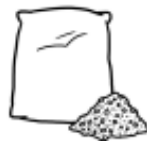
Washed drainage gravel (6-12mm)
