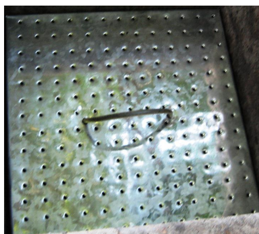
Holes should be 3mm diameter, 2.5 cm (1") apart.
