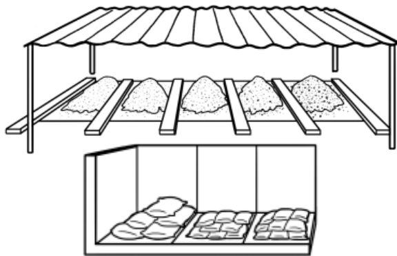
Storage areas for sieved and washed/bagged sand
